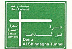
Direction signs showing the shape of junction ahead and indicating routes and places extending from it
